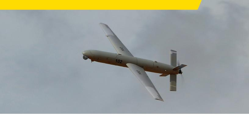
SkyStriker is a fully autonomous loitering munitions (LM) that can locate, acquire and strike operator-designated targets with a 5 or 10 Kg warhead installed inside the fuselage, enabling high-precision performance.
